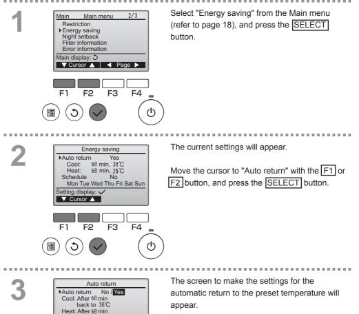
Move the cursor to the desired item with the F1 or F2 button out of "Auto return," "Cool," or "Heat."
